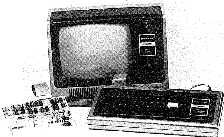
Fig. 6-1. TRS-80 computer and breadboard in experimental use position.
